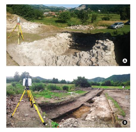
Pic. 1. Bologa, fort Resculum. Instruments used for scanning A – Leica Viva MS60 (year 2016), B – HDR Leica ScanStation P50 (year 2017) (Photo: T. Górzyński)
