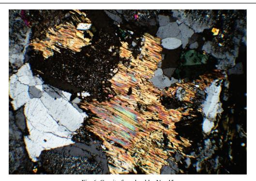
Fig. 6. Granite from boulder No. 45 visible crystals of K-feldspar, quartz and colourful lamellae of biotite; polarising microscope, PolaroidX, magnification 40×
