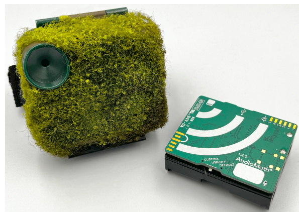
Fig. 1. AudioMoth deployment package in a customized protective casing (photo by M. Adamiak 2024)
