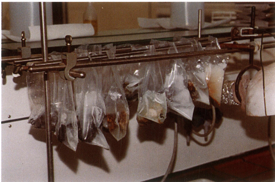
Pl. 1. Refrigerator in which the experiment was carried out. Plastic bags with rock samples were immersed into solution of non-freezing liquid
