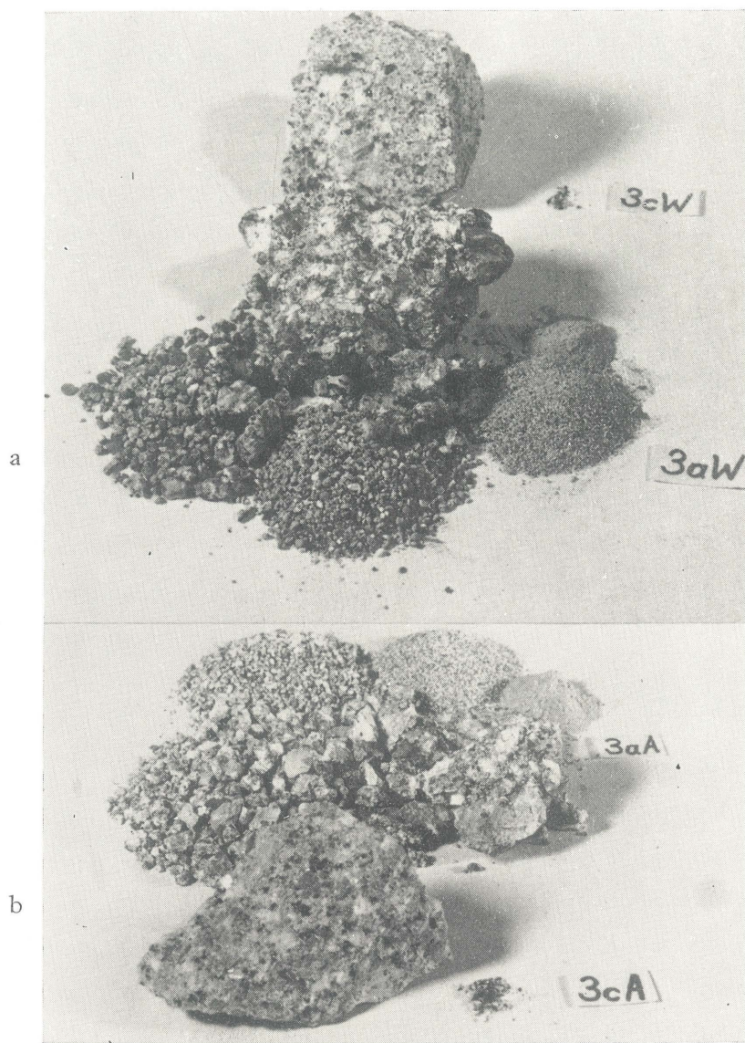
Pl. 1. Porphyrocrystic granite (Jelenia Góra) strongly weathered from the waste cover surface (3a) and fresh from a quarry wall (3c)
