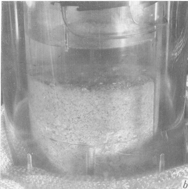
Pl. 7. Top (a) and side (b) view of "inverted open system" cabinet showing a5-2 sample at cycle 1, freezing at a rate of 0.6 mm/hr
