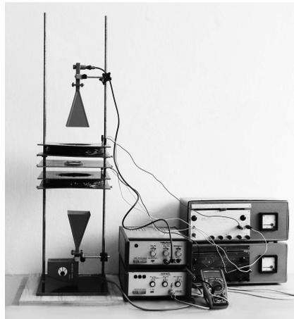
Photo 1: External view of the system, where absorption of waves in ferrofluids was investigated.
