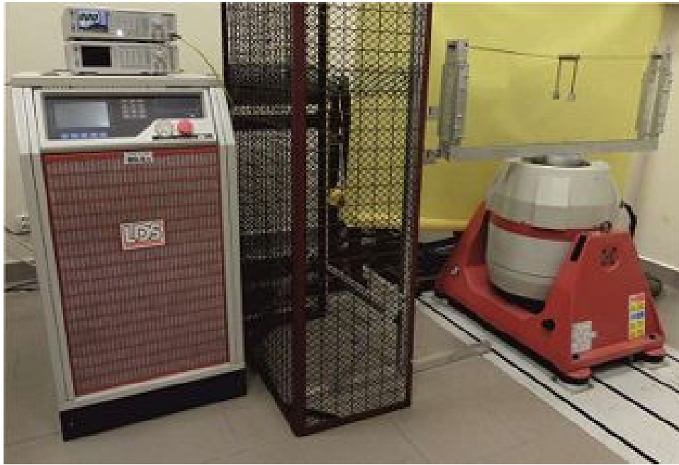
Fig. 5: An experimental rig consisting of the beam with pendulums mounted on the electrodynamic shaker.
