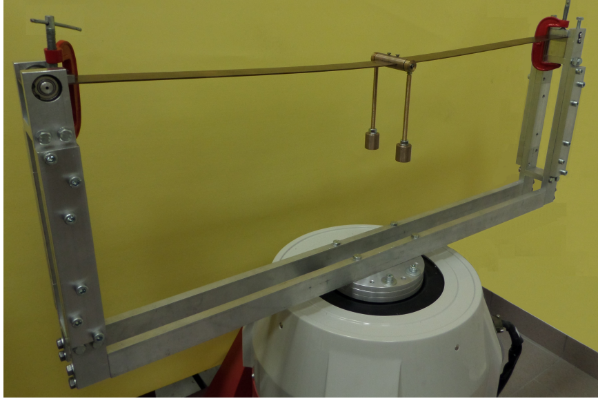
Fig. 6: Experimental rig consisting of one oscillator node ( n = 1 ).
